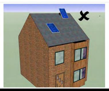
Solar panels should be evenly positioned and fitted flush with the roof slope and should not protrude above the ridge height.
